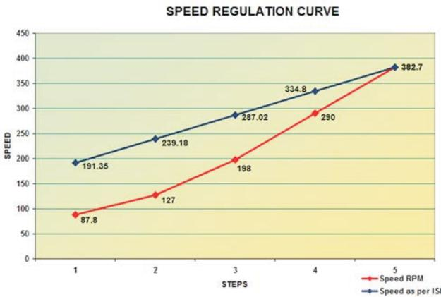
Type C fan tested on a standard regulator
