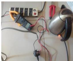
**K:** Electric kettle current measurement
