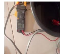
**M:** Electric boiler current measurement.
