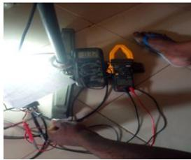
**A:** Electric fan voltage and current measurement
