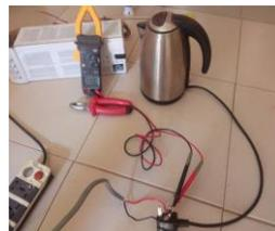
**J:** Electric kettle voltage measurement.
