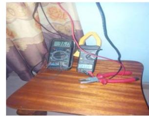
**D:** 1Hp AC voltage and current measurement
