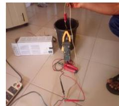
**L:** Electric boiler voltage measurement.
