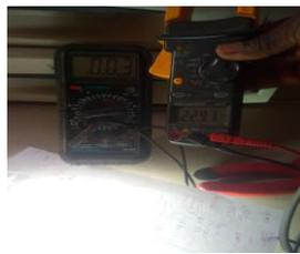
**B:** Lighting point voltage and current measurement
