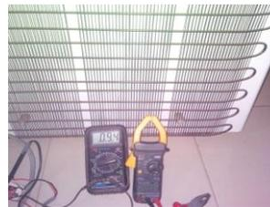
**G:** Refrigerator voltage and current measurement
